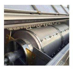
filter screen. The drum rotates slowly, and the backwash pump draws filtered water to backwash the filter screen. The washed dirt falls into the collection tank inside the drum and is discharged outside the equipment through the blowdown pipe.
